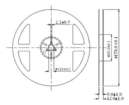
Unit: mm Tolerance:  $\pm 0.25$ mm
